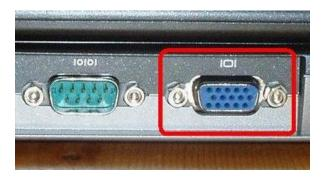
This is the monitor out connector on the back panel of a Dell Latitude D520. The connection on a PC is identical.
